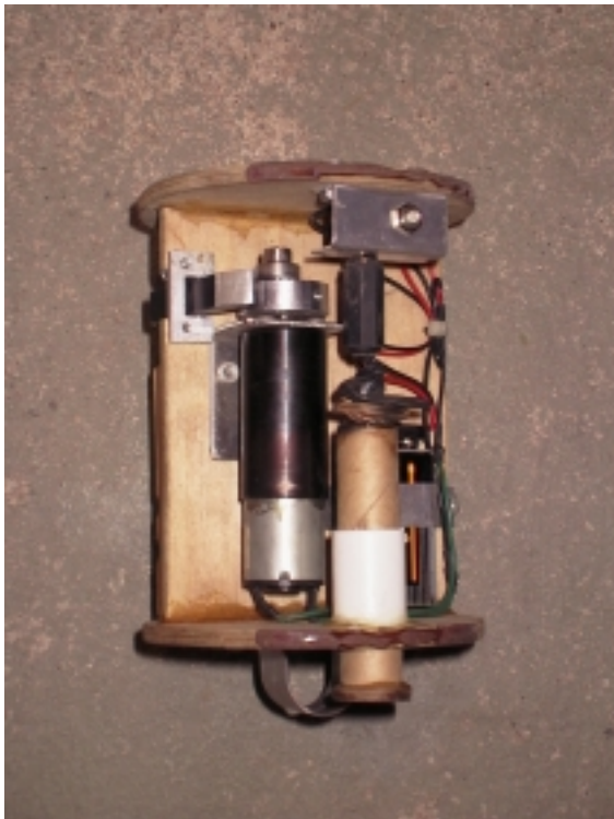
Various views of the rocket camera showing the gear motor, cam, and lever. The cardboard tube in the center is a lead weight for pulling the plug from the headphone jack.
